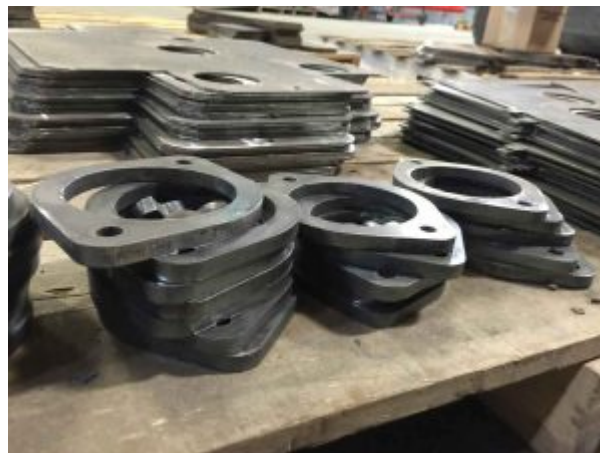
Parts cut using both waterjet and plasma technologies.
