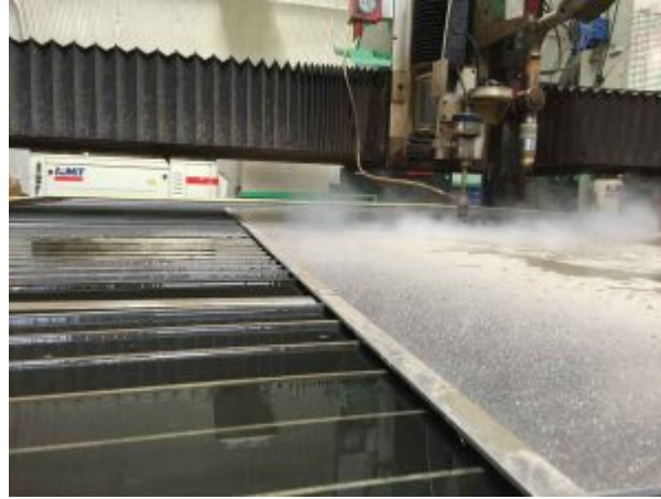
The waterjet cutting system in action on the Machitech combination table.
